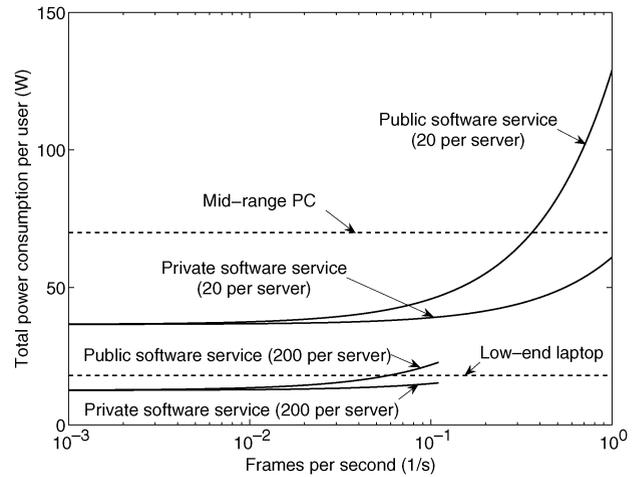
**Fig. 7. Per-user power consumption of public and private cloud software services as a function of download rate. Also included is the power consumption of a low-end laptop and the power consumption at idle of a modern midrange computer.**
