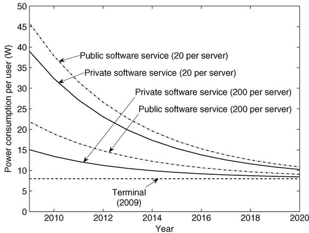
**Fig. 12.** Per-user power consumption of public and private cloud software services with 20 and 200 users per server for the years 2009–2020. Also included is the power consumption of a user terminal from 2009.
