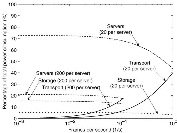
**Fig. 6. Percentage of total power consumption of transport, storage, and servers of a private cloud storage service as a function of download rate with 20 and 200 users per server. The percentage of total power consumed by the user terminal is not shown.**
