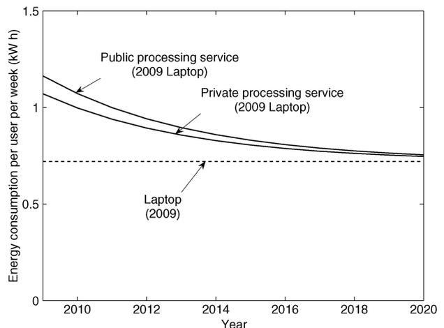
**Fig. 13.** Per-user per-week energy consumption of public and private cloud processing services for the years 2009–2020. The cloud processing service is used to perform an average of 0.5 encodings per week. The total energy consumption includes the energy consumed in the user’s laptop. Also included is the power consumption of a 2009 low-end laptop.
