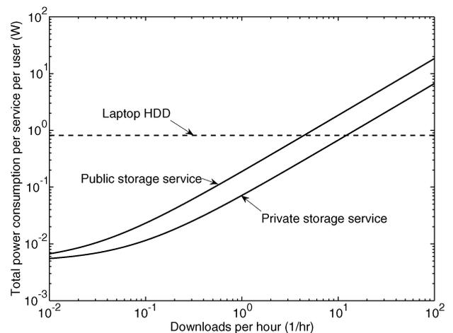
**Fig. 4. Per-user power consumption of public and private cloud storage services as a function of download rate. Also included is the power consumption of a modern laptop HDD. The average document size is 1.25 MB.**
