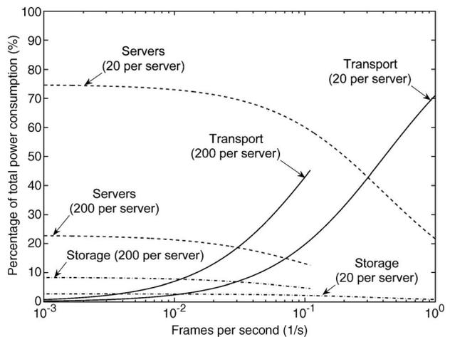
**Fig. 5. Percentage of total power consumption of transport, storage, and servers of a public cloud storage service as a function of download rate with 20 and 200 users per server. The percentage of total power consumed by the user terminal is not shown.**
