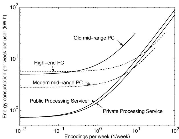
**Fig. 10. Power consumption of public and private cloud processing services as a function of encodings per week. Also included is the power consumption of a modern midrange PC and the power consumption of a modern idle of a high-end PC.**
