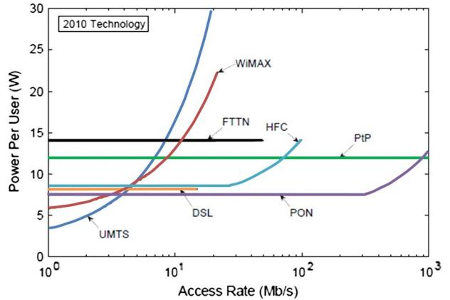
**Fig. 7. Power per user for access network technologies as a function of access rate. Although wireless access is relatively energy efficient at very low rates, it becomes the least efficient as rates increase. PON provides the most energy-efficient access technology for rates less than around 1 Gb/s. Note that these comparisons are based upon 2010 technologies.**
