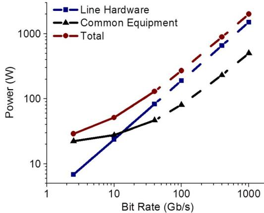
**Fig. 3.** Capacity-dependent optical line card power. Values beyond 40 Gb/s are extrapolated following the logarithmic trend.
