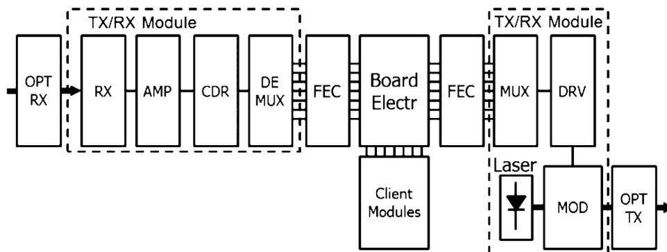
Fig. 2. Transceiver line card model for on-off keyed modulation.
