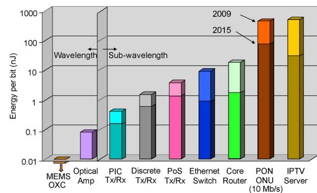
**Fig. 5. Energy per bit of different types of network elements.**
