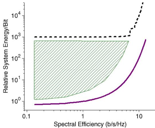
**Fig. 4.** System efficiency (dashed) and the ideal Shannon limited efficiency (solid). Hatched area shows region for potential efficiency improvements.
